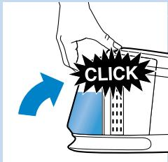
**4** Refill the water tank and reattach it to the steam generator.
