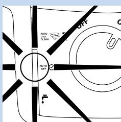
*Note: If you do not use the iron for more than 10 minutes, the appliance switches off automatically for safety reasons. The automatic shut-off light flashes. To switch on the appliance again, press any button.*
