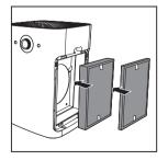
5 After the pre-filters are properly put back in the appliance, reset the filter lifetime counter. (Refer to chapter 7 "Resetting the filter lifetime counter".)
