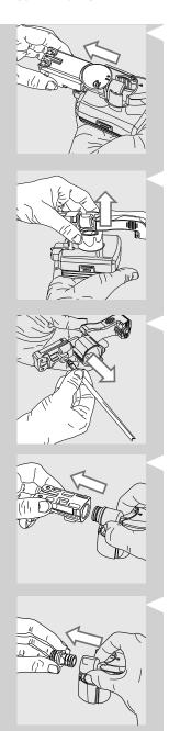
5 Remove the connector which is in contact with the machine.
