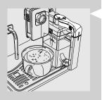
4 The machine starts pouring hot milk. The pouring can be stopped earlier by pressing the "\" button.
