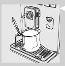
16 Place a container under the dispensing spout to catch the small amount of water which will be dispensed.
