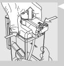
2 Press the release buttons and lift the lid.
