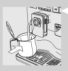
5 When the dispensing has finished, empty the container and place it under the hot water/steam wand.
