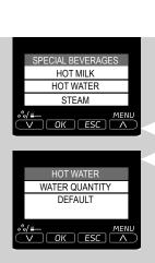
2 Select HOT WATER by pressing the "√" or "∧" scrolling button. Press "OK" to confirm.
