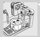
9 Remove the cup and close the milk dispenser by turning it counter clockwise.
