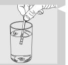
1 Immerse the water hardness test strip provided with the machine in water for 1 second.
