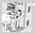
13 Remove the milk carafe and the container from the machine.
