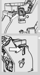
9 Make sure the hook to lock the brew group is in the correct position by firmly pressing the "PUSH" button until you hear a click. Check if the hook is at the top end position. If it is not, please try again.
