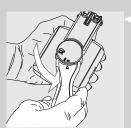
4 Rotate the handle counter-clockwise to the unlock position up to the "
