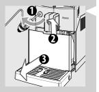
16 To clean the drip tray, place a "Coffee Oil Remover" tablet inside and fill it 2/3rds full with hot water. Let the cleaning solution take effect for about 30 minutes, then rinse thoroughly.
