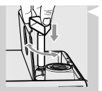
While the machine grinds coffee, press and turn the grinder adjustment knob placed inside the coffee bean hopper one notch at a time. Use the special coffee grinder adjustment key supplied. You will taste the difference after brewing 2-3 cups of coffee.
