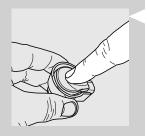
**22** Reassemble the lid making sure that you press it in the middle to have it correctly inserted.
