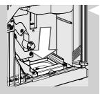
14 Insert the coffee residues drawer into its seat and ensure that it is correctly in place.
