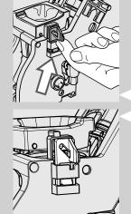
13 Make sure that the hook which locks the brew group is in the correct position. If it is still in the downward position, push it upward until it locks correctly into place.
