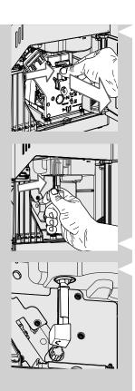
4 To remove the brew group, press the «PUSH» button and pull it by the handle. Pull it out horizontally without turning it.
