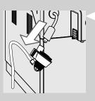
**16** Remove the chrome cover with the rubber fitting from the steam wand.
