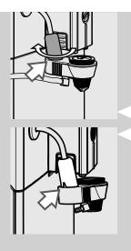
18 Make sure that it is positioned correctly. If you cannot insert it, rotate the chrome cover. The Automatic Milk Frother is assembled correctly when the tooth fits into the slot.
