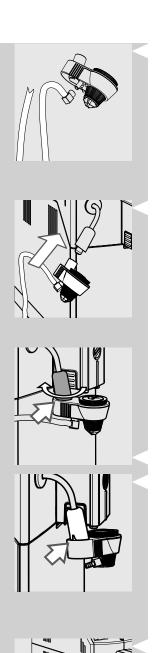
3 Insert the suction tube into the Automatic Milk Frother.
