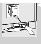
12 Switch the power button to "I". The "(|)" button flashes.
