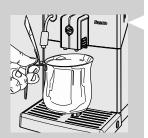
During this process the coffee brewing cycle is activated and fresh water flows through the water circuit. This takes a few minutes.
