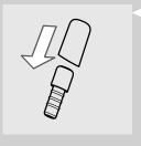
25 Insert the rubber fitting into the chrome cover.
