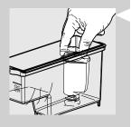
16 Remove the small white filter and place the "INTENZA+" water filter into the water tank if it was installed.
