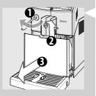
15 The machine warms up and performs the automatic rinse cycle. Remove and empty the container. Empty the drip tray and place it back.
