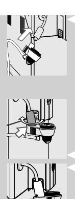
27 Insert the Automatic Milk Frother in the rubber fitting.
