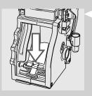
111 Gently pull down the lever until it is in contact with the brew group base and the two reference marks on the side of the brew group match.
