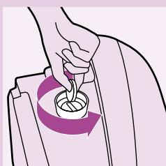
**4** Turn the steam tank on its side and remove the Calc-Clean rinsing cap & rinsing plug with the special key supplied or with a coin.
