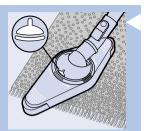
4 With the nozzle positioned lengthwise and the brush strip folded in, you can vacuum clean small soft floor areas. Turn the nozzle 90 degrees clockwise again until it is positioned lengthwise with the brush strip still folded in.
