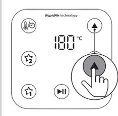
3 Press the up or down button to choose the needed temperature.
