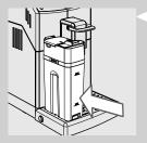
**2** Fill the milk carafe with water up to the MIN level and insert it into the machine.
