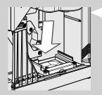
14 Insert the coffee residues drawer in its seat and ensure that it is correctly in place.
