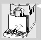
4 Insert the coffee grounds drawer back into the drip tray and place the drip tray back into the machine.
