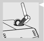
3 Lift the pre-ground coffee compartment lid and add one level measuring scoop of pre-ground coffee. Use only the measuring scoop supplied with the machine. Then close the pre-ground coffee compartment lid.
