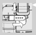
3 Insert the carafe into the machine. Pull out the milk carafe dispenser to the right up to the " 📥 " icon.
