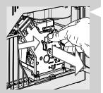
**4** To remove the brew group, press the «PUSH» button and pull it by the handle. Pull it out horizontally without turning it.
