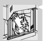
After rinsing the brew group, insert it back into its seat until it locks into place (see the "Weekly Cleaning of the Brew Group" chapter). Insert the drip tray and the coffee grounds drawer. Close the service door.
