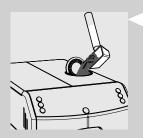
3 Lift the pre-ground coffee compartment lid and add one level measuring scoop of pre-ground coffee. Use only the measuring scoop supplied with the machine. Then close
