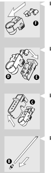
10 Insert the fitting (F) into the milk frothing device by pressing it up to its limit.
