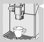
2 Place a cup under the dispensing spout. Press the " $\underbrace{P}_{MEMO}$ " button to brew an espresso.
