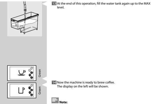
The automatic rinse/self-cleaning cycle starts when the machine has been in stand-by mode, or turned off, for more than 15 minutes. When you have not used the machine for 2 or more weeks, you will also need to perform a manual rinse cycle. At the end of the cycle, you can brew a coffee.
