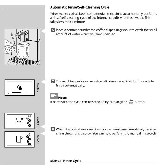
During this process, the coffee brewing cycle is activated and fresh water flows through the water circuit. This takes a few minutes.
