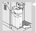
Push the carafe towards the bottom while rotating it at the same time, until it is locked onto the drip tray. Do not force the carafe while inserting it.
