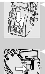
Gently pull down the lever until it is in contact with the brew group base and the two reference marks on the side of the brew group match.
