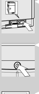
12 Switch the power button to "I". The "(1)" button flashes.
