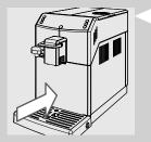
**16** Insert the coffee grounds drawer with the drip tray back into the machine and close the service door.
