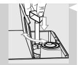
4 The reference marks inside the coffee bean hopper indicate the grind setting. There are 5 different grind settings to choose from, from position 1 (●) for coarse grind - lighter taste to position 2 (•) for fine grind - stronger taste. If coffee is watery or is brewed slowly, change the coffee grinder settings.
