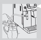
2 Insert the other end of the suction tube into the milk container.
