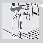
5 Remove the suction tube that is installed in the Cappuccinatore.
