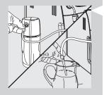
2 Insert the suction tube in the milk container or into the milk thermos.
