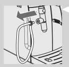
1 Remove the pin with the suction tube from the Cappuccinatore.
