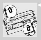
4 To remove the tray, press on the hooks on the bottom of the coffee bean hopper as shown in the figure above.
