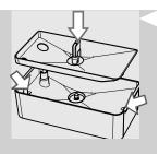
6 After cleaning, insert the tray back into the coffee bean hopper. Insert the tray hooks into their seats on the coffee bean hopper.
