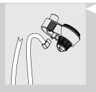
1 Insert the suction tube into the Automatic Milk Frother.
