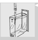
15 Rinse the water tank and fill it with fresh water up to the MAX level. Put it back into the machine. Repeat step 13.
