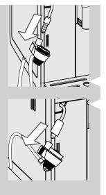
2 Remove the Automatic Milk Frother from the steam/hot water wand.
