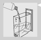
4 Remove the "INTENZA+" water filter (if any) from the water tank and replace it with the small white original one. Pour all the descaling solution into the water tank.
