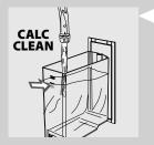
5 Fill the water tank with fresh water up to the CALC CLEAN level and put it back into the machine.
