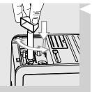
2 Press and turn the grinder adjustment knob inside the coffee bean hopper one notch at a time. Use the special coffee grinder adjustment key supplied. You will taste the difference after brewing 2-3 cups of coffee.
