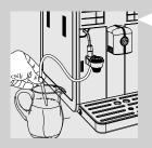
10 Insert the suction tube into the container.
