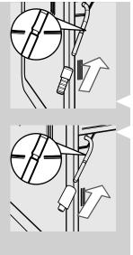
27 Insert the rubber fitting back and the chrome cover (if any) on the steam wand.
