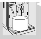
6 Place a large container (1.5 l) under both the steam/hot water wand and the coffee dispensing spout.
