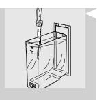
10 Rinse the water tank and fill it with fresh water up to the MAX level. Put it back into the machine.
