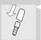
26 Insert the rubber fitting into the chrome cover (only for Automatic Milk Frother with chrome cover).
