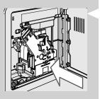
12 After rinsing the brew group, insert it back into its seat until it locks into place (see the "Weekly Cleaning of the Brew Group" chapter). Insert the coffee residues drawer and the coffee grounds drawer. Close the service door.
