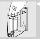
20 Remove the small white filter and place the "INTENZA+" water filter into the water tank if it was installed.
