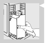
6 Remove the water tank by pulling it by the handgrip.
