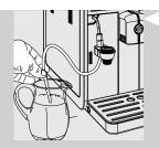
3 Insert the suction tube into the milk container.
