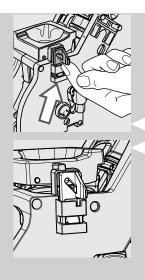
12 Make sure that the hook which locks the brew group is in the correct position. If it is still in the downward position, push it upward until it locks correctly into place.
