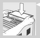
4 Insert the coffee bean hopper into its compartment as shown in the figure.
