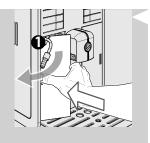
5 Press gently on the side of the water tank door to release the handgrip.
