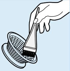
**3** Clean the sieve by means of the brush supplied.
