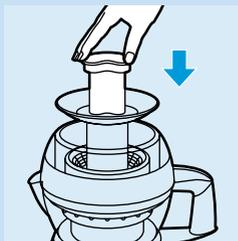
The appliance will only function if the jug and the lid have been properly mounted onto the motor unit.
