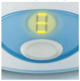
The display and sound alerts tell you when sterilisation is complete and how long items will remain sterile. The display also lets you know when you have filled the steriliser with too little or too much water, so you can always be sure that sterilising has been completed accurately and reliably.
