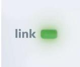
Indicates a continuous connection between the baby and the parent unit with visible and audible link indicators.
