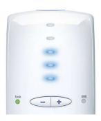
Lights are activated to indicate the level of sound in your baby's room, even if the volume is off
