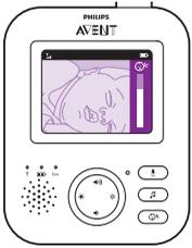
If your baby only makes soft sounds, the sensitivity of the baby unit needs to be set to a high sensitivity level on the parent unit.
