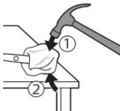
Note: You may have to hit on the end several times to break the internal snap connections.
