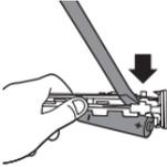
7 Wedge the screwdriver between the battery and the black frame at the bottom of the internal components. Then pry the screwdriver away from the battery to break the bottom of the black frame.
