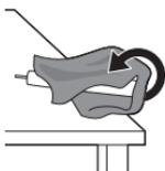
**3** Hold the top of the handle with one hand and strike the handle housing 0.5 inch above the bottom end. Strike firmly with a hammer on all 4 sides to eject the end cap.
