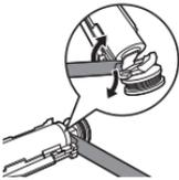
8 Insert the screwdriver between the bottom of the battery and the black frame to break the metal tab connecting the battery to the green printed circuit board. This will release the bottom end of the battery from the frame.
