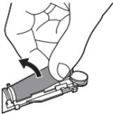
9 Grab the battery and pull it away from the internal components to break the second metal battery tab.
