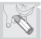
9 Pry the 2 AA-sized cylindrical nickel metalhydride batteries loose by inserting the screwdriver on the sides of the two batteries in the locations shown in the figure.
