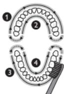
The Quadpacer is an interval timer that has a short beep and pause to remind you to brush the 4 sections of your mouth. Depending on the brushing mode you have selected, the Quadpacer beeps at different intervals during the brushing cycle. The Quadpacer works in all 5 modes.
