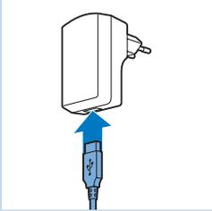
**1** Insert the standard USB plug into the socket of the adapter.
