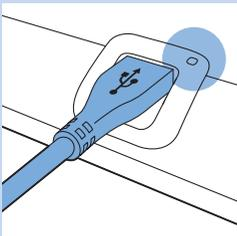
**4** When the battery is fully charged, the charging light turns solid green.
