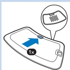
The BlueTouch Pain Relief Patch has three modes and an 'off' setting (see chapter 'Treatment schedule and treatment modes'). Press the mode button one or more times to select one of the three treatment modes. When you press the mode button a fourth time, you switch off the BlueTouch Pain Relief Patch.
