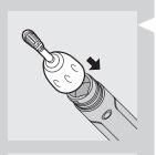
1 Align the front of the brush head with the front of the toothbrush handle. Match the bars that are on the inside top of the removable nut with the notches inside the top of the handle and slide the brush head onto the handle.
