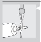
1 Remove the brush head and rinse the metal shaft area with warm water.
