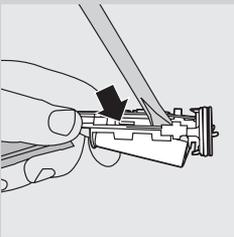
**4** Insert the screwdriver under the circuit board, next to the battery connections, and twist to break the connections. Remove the circuit board and pry the battery from the plastic carrier.
