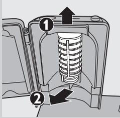
**4 Remove the protective screen in front of the UV light bulb.**
