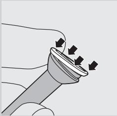
**2** Install a new ring by slipping one edge of the new ring over the bottom of the brush head. Then press down on the other side to snap the ring in place.
