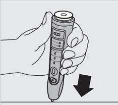
**3** Hold the handle upside down and push down on the shaft to release the internal components of the handle.
