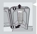
4 Remove the protective screen in front of the UV light bulb.
