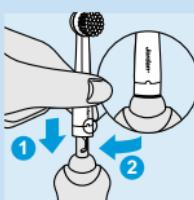
**3** Mount the brush head on the toothbrush by inserting it into the bayonet catch and turning it.
