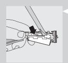
Insert the screwdriver under the circuit board, next to the battery connections, and twist to break the connections. Remove the circuit board and pry the battery from the plastic carrier.
