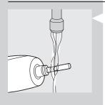
1 Remove the brush head and rinse the metal shaft area with warm water.
