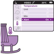
2 In the temperature menu, an alert for temperature can be set on or off.
