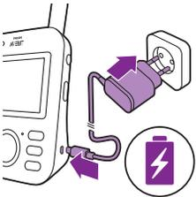
The parent unit runs on a built-in rechargeable Li-ion battery.
