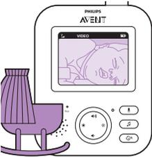
When the VIDEO mode is activated, the screen is always on, so you can see your baby. All sounds are directly transmitted to the parent unit.
