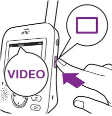
Press the mode button on the side of the parent unit to select the VIDEO mode.
