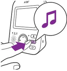
1 Press the lullaby button on the parent unit to open the menu for lullabies. Press the left part of the control button and then press the bottom of the control button to select the volume options of the lullaby menu. Press the right part of the control button to access the lullaby volume levels.
