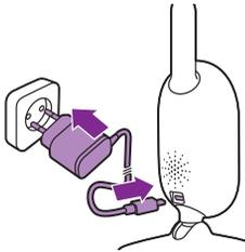
Put the power adapter in the baby unit and the adapter in the wall socket.
