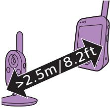
3 Make sure that the parent unit and the baby unit are at least 2.5 meters/ 8.2 feet away from each other to avoid acoustic feedback.
