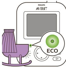
When sound is picked up by the baby unit, the display and sound of the parent unit switch on immediately. The sounds are transmitted to the parent unit.
