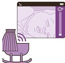
If your baby only makes soft sounds, the sensitivity of the baby unit needs to be set to a high sensitivity level on the parent unit.
