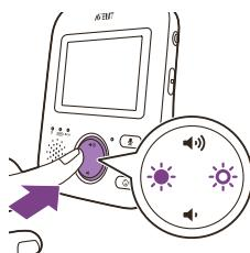
You can adjust the display brightness of the parent unit to the level you prefer.
