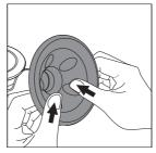
4 Put the silicone diaphragm onto the pump body and press the rim to make sure a perfect seal.
