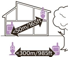
The operating range is up to 50 meters / 165 feet indoors and 300 meters / 985 feet outdoors. The operating range of the baby monitor varies depending on the surroundings and factors that cause interference. Wet and moist materials cause so much interference that the range loss is up to 100 %.
