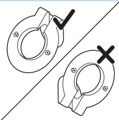
**Note:** Make sure that the ring of the wall mounting bracket slants downward when you hold it to the wall. If the ring of the wall mounting bracket slants upward, turn the wall mounting bracket the other way around so that it is in the correct position.
