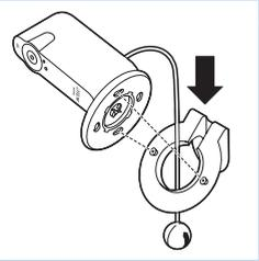
6 Pass the humidity and temperature sensor unit through the hole in the wall mounting bracket. Then align the slots in the foot of the baby monitor with the projections on the ring. Fit the groove in the foot of the baby monitor onto the raised edge on the inside of the ring.
