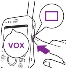
When the VOX mode is activated, the display and sound of the parent unit switch off, if there is no sound detected for 20 seconds.
