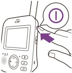
4 Press the on/off button on the parent unit to switch on the parent unit.
