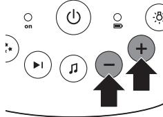
Note: You can only set the loudspeaker volume on the baby unit when a lullaby is playing. If you set the volume for the lullaby higher, the sound will also be louder when you use the talk function on the parent unit.
