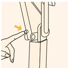
The appliance fails to unlock automatically. In that case you first have to press unlocking button (B), after which you can fold the appliance back into its transport position in the manner indicated in the chapter 'Storage'. If the appliance fails to unlock several times, contact your dealer or a Philips service centre.
