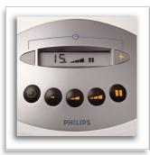
Treatment time can easily be controlled by setting the advised or preferred number of minutes. The digital timer automatically counts down and automatically shuts off at the end of the session.
