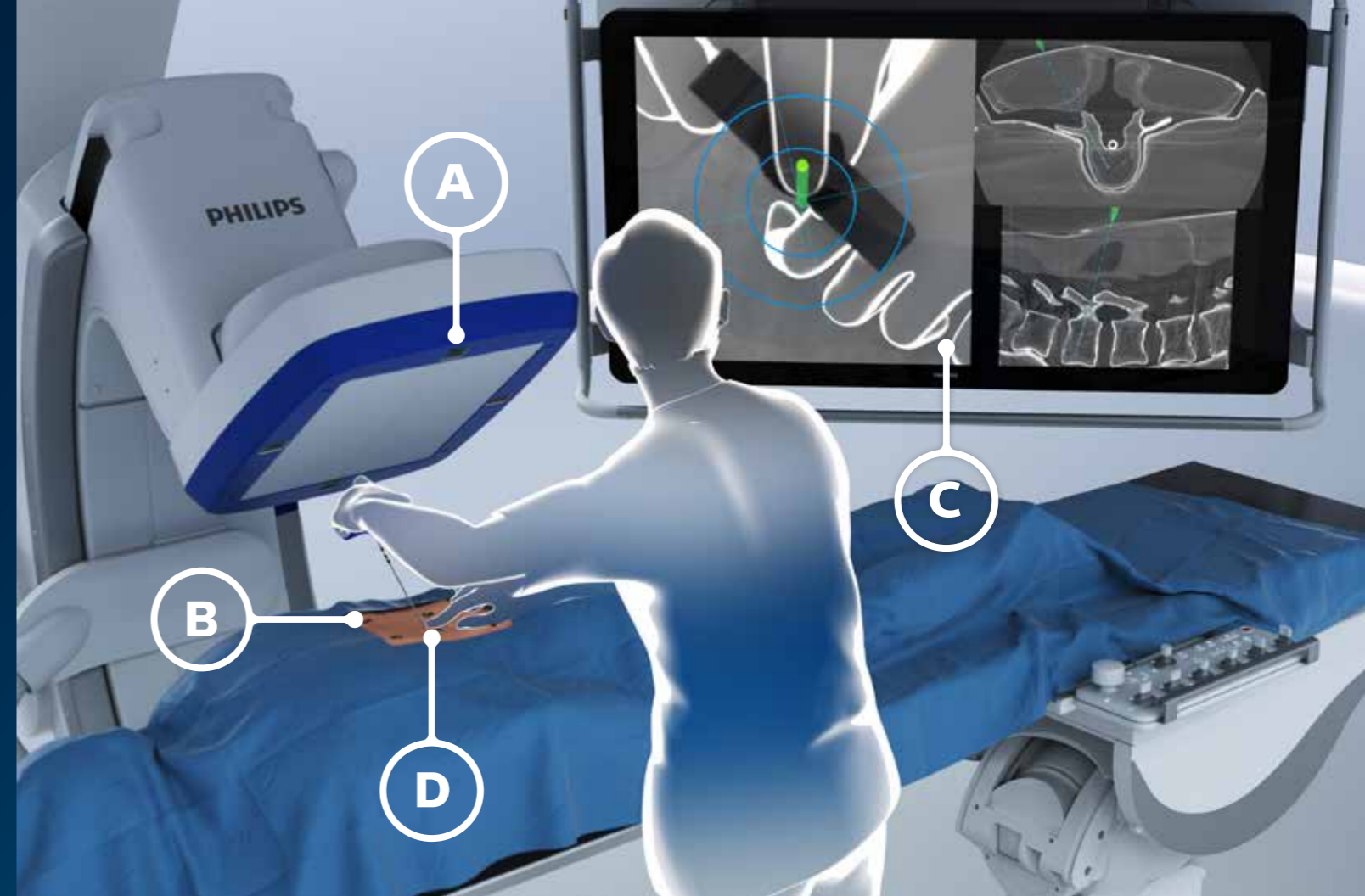
Four high-resolution cameras in the C-arm Flat Detector (A) automatically detect the non-invasive patient markers (B) to augment the surgical field. The live video images provided by the cameras are overlaid on 3D cone-beam CT (C) The systems visualizes the tip of the ClarifEye Needle as it is navigated along the planned path on the spinal anatomy (D).
