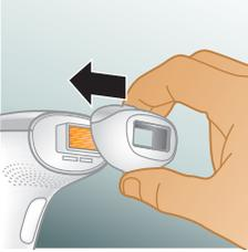
To place the attachment, simply snap it onto the light exit window.
