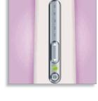
Press the intensity increase/decrease button up or down to change the intensity (from 1 to 5). The corresponding intensity light starts to flash.
