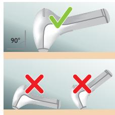
2 Place the device at a 90° angle on the skin so that the attachment and the safety ring are in contact with your skin. The safety ring prevents unintentional flashing without skin contact.
