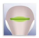
6 Press the safety ring fully onto the skin with slight pressure. When all contact switches of the appliance are in contact with the skin, the "ready to flash" light on the back of the appliance lights up green.
