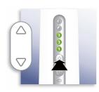
4 Press the intensity increase/decrease button up or down to change the intensity (from 1 to 5).
