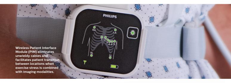
The ST80i has a compact wireless patient module that sets it apart from traditional stress-testing systems. The wireless module reduces the hazard of tripping over wires and enhances patient comfort and movement.
