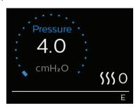
Your device has two ramp modes. Your provider will select the one that is most appropriate for you. The standard ramp mode increases pressure at a steady rate. Alternately, the SmartRamp mode maintains a constant lower pressure until the device detects that you require more pressure.
