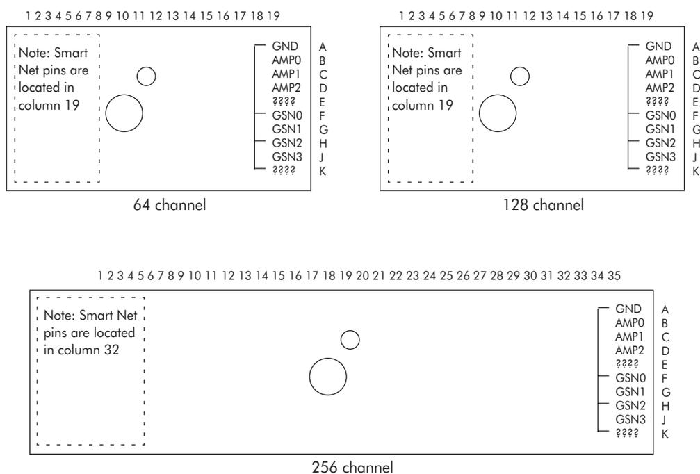
**Figure 8-6.** Schematic view of GSN connectors
