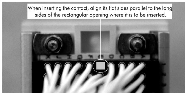
**Figure 9-13.** View of connector before inserting contact
