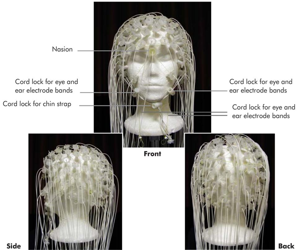
**Figure 3-3.** GSN 200 (128-channel model), without wire management
