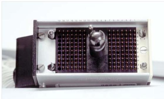
**Figure 8-2.** Hypertronics plug of 128-channel GSN
