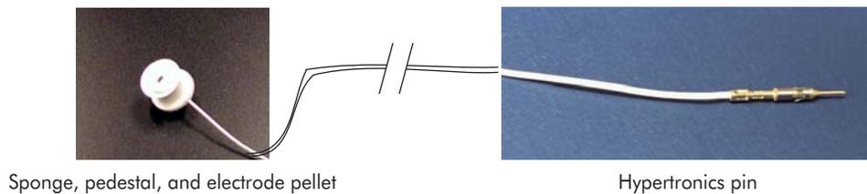
**Figure 2-7.** Sensor connected by wire to pin
