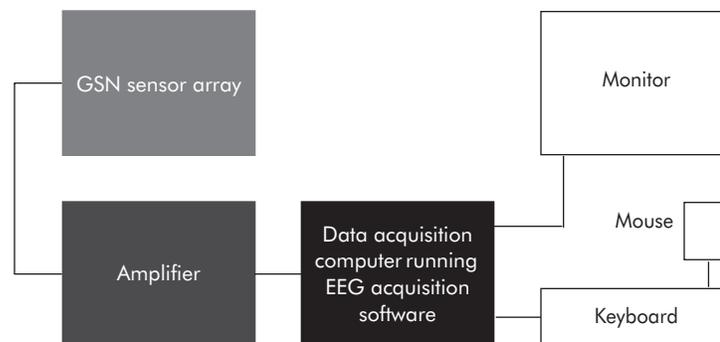
**Figure 1-4.** Functional block diagram of a typical GES
