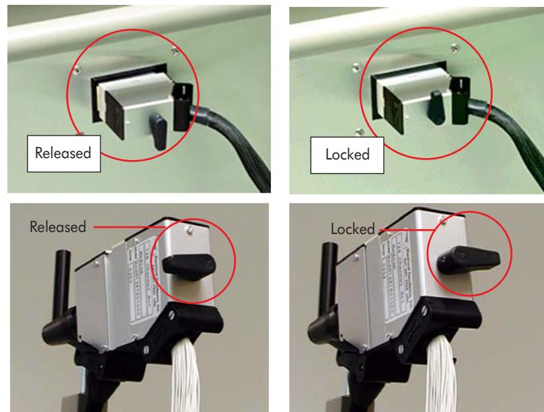
**Figure 8-3.** Hypertronics plug released (left) and locked (right)
