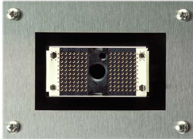
**Figure 8-1.** Multicontact Hypertronics receptacle (128-channel Net Amps 200 amplifier)
