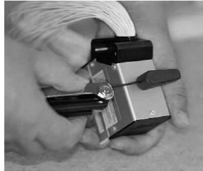
**Figure 9-3.** Remove the handle on the Hypertronics plug
