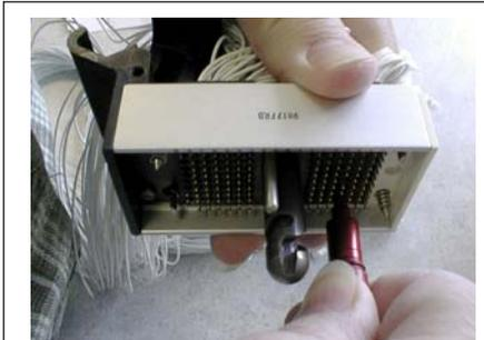
**Figure 9-10.** Push the tool until the contact pin slides out
