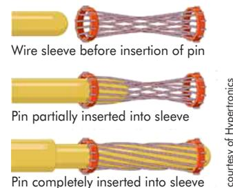
**Figure 8-4.** Magnified view of Hypertac pin and sleeve
