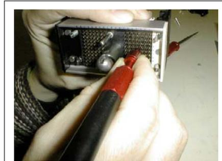
**Figure 9-9.** Remove the contact using the extraction tool
