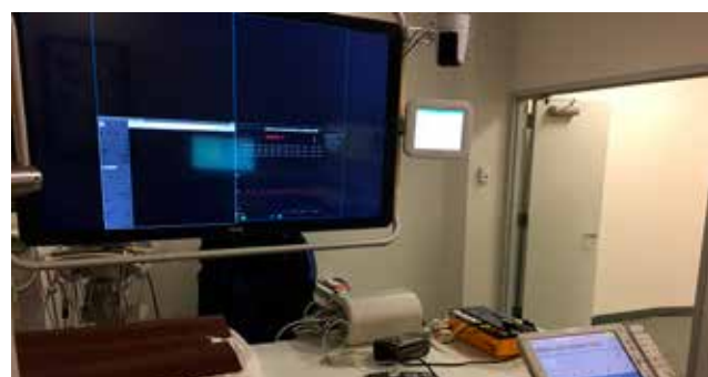
Test set-up in an exam room showing the exam room user interface, TSM workspot, FC2010 monitoring device and Fluke Vital Signs patient simulator.
