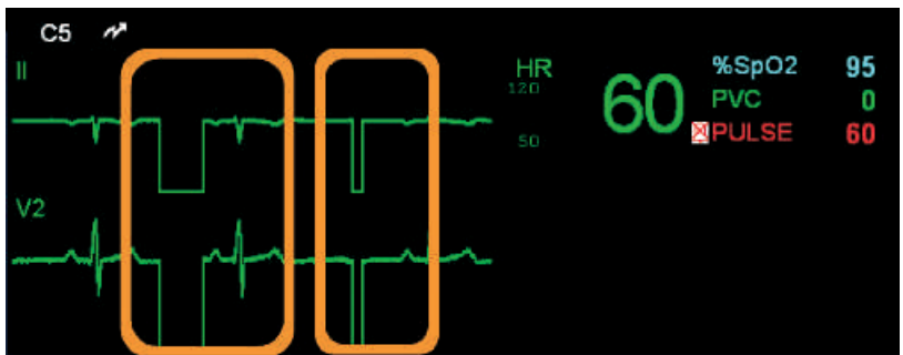
Data dropouts in sample telemetry waveform display.
