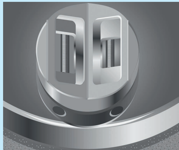
Cathode head with two filaments of a double focus tube
