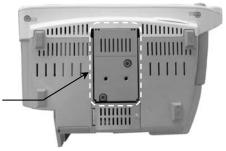
1. Fasten the Table Top Mount to the Mounting Adapter with one (1) M6 x 12mm FHMS and two (2) M6 x 8mm FHMS as shown below.
