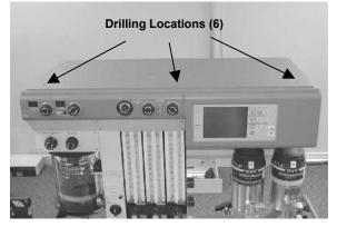
Loosen the socket set screws (2 each side) to release the top of the machine. Lift up on the top of the machine and drill in the locations marked in step #1. Use a ¼" diameter drill bit. Be careful not to drill too deeply, as damage to internal components of the machine could result. Remove all drilling chips.
