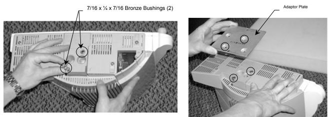
2. Secure the Adaptor Plate to the device by using the supplied M6 x 40mm FHMS (2).
