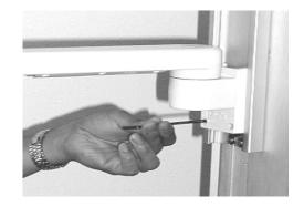
2. Align the screw holes in the Down Post with the threaded holes on the Swivel Fitting. Using the supplied 5/32 (4 mm) hex key and secure the 10-32 x 3/8" SHCS (3).
