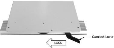
2. To prevent the Camlock Lever from being unlocked, insert one (1) #6-32 x 3/8" PHMS in the threaded hole to the right of the Lever (below right). To further secure the Camlock Mount in the Rails, insert one (1) M4 x 20mm PHMS in each of the two (2) threaded holes at the rear corners of the Mount (below right). Stop tightening these screws when they make contact with the bottom of the Rail.
